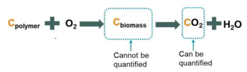
As you can see  $CO_2$  evolution is related to the biodegradation of the polymer, therefore by analysing the evolved  $CO_2$  throughout the test it is possible to extrapolate the biodegradation of the film at different gauges over time.
