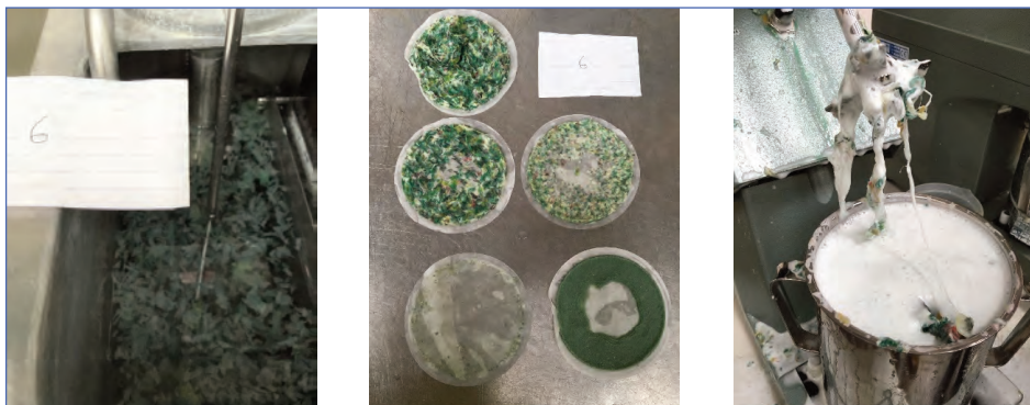
Figure 9 Sample ref. 17 High solids (27.6%) > 2.38mm retained by Mesh 8 filter in Bauer McNett (left) and recovered on Mesh 8 filters (middle – top left). Sample 21 – trial discontinued due to presence of non-repulpable 'strings' on impeller and excessive pulper losses (right)
