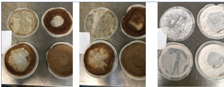
Figure 8 Non filtrable solids retained for Recycled liner with solvent free adhesive (1) (sample ref. 5 – left), Recycled liner with solvent free adhesive (1) and Hydropol film (sample ref. 6 – middle) and kraft (100gsm) with solvent free adhesive (1) and Hydropol film (sample ref. 15 – right). Each picture shows retained solids by mesh 8 (top left), mesh 16 (top right), mesh 50 (bottom left) and mesh 100 (bottom right)
