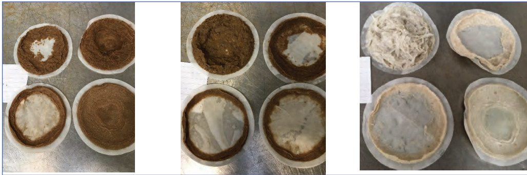
Figure 10 Non-filtrable solids retained for Recycled liner with – (left), Recycled liner with solvent based adhesive and Hydropol film (sample ref. 8 – middle) and newsprint (40 gsm) with solvent based adhesive and Hydropol film (sample ref. 18 – right). Each picture shows retained solids by mesh 8 (top left), mesh 16 (top right), mesh 50 (bottom left) and mesh 100 (bottom right)
