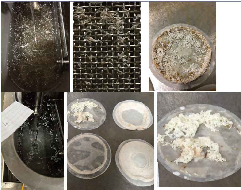
Figure 11 Sample ref 5 - sticky threads > 2.38mm retained by Mesh 8 filter in Bauer McNett (top left) and adhering to mesh 8 screen (top middle). Stickies retained on Mesh 8 filter paper (top right). Sample ref 16 – sticky threads retained by mesh 8 filter in Bauer McNett (bottom left) and presence of stickies on mesh 8 filter paper (bottom middle and right)
