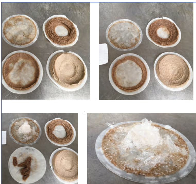
Figure 6 Non filtrable solids retained for White Top (sample ref. 12 – top left), White Top/water-based repulpable adhesive/Hydropol film (sample ref. 13 – top right), White Top/water-based repulpable adhesive and Hydropol/polyethylene coextrusion film (sample ref. 14 – bottom left) and mesh 8 non-filtrable solids showing high quantities of retained PE. Each picture shows retained solids by mesh 8 (top left), mesh 16 (top right), mesh 50 (bottom left) and mesh 100 (bottom right)
