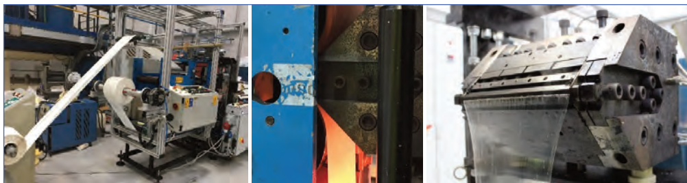
Figure 3 Pilot extrusion coating line showing base-paper unwind and coated paper rewind (left), extrusion die applying a Hydropol polymer to paper (middle) and extrusion die extruding Hydropol polymer curtain (right)
