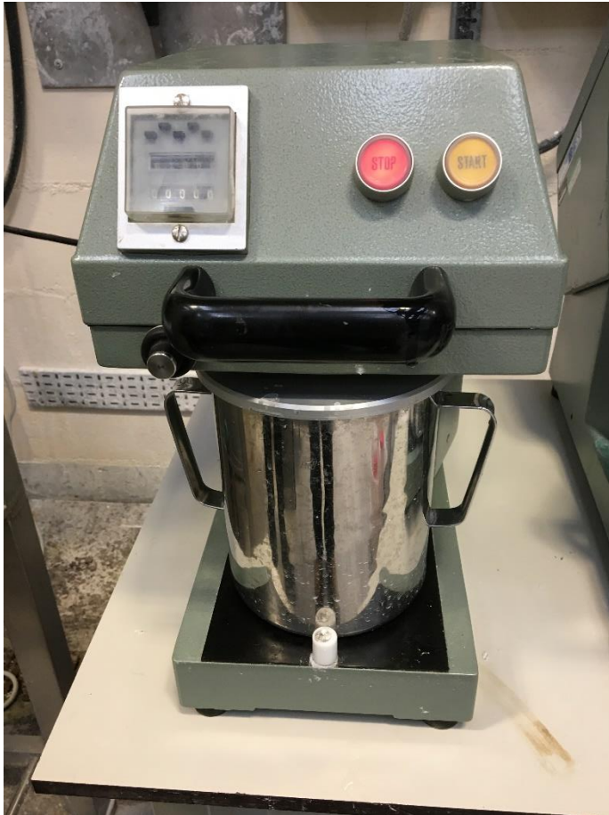
Laboratory disintegrator, temperature checks and charging pulper with test sample
