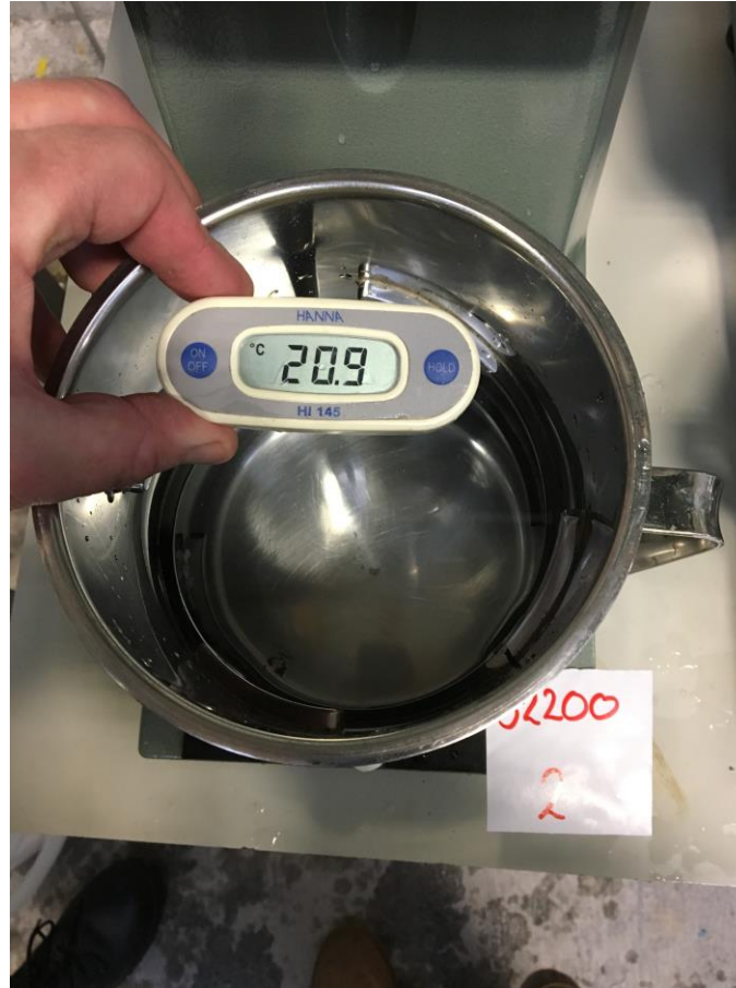
Laboratory disintegrator, temperature checks and charging pulper with test sample
